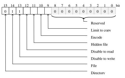
"Limit to copy" - This bit enable/disable to limit number of times for copy. If it is 1, copy is allowed within number specified in CC(Copy Counter). This bit is only for RAM area so that this should be set with "0" in ROM area.
