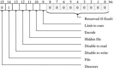
"Limit to copy" - This bit enable/disable to limit number of times for copy. If it is 1, copy is allowed within number specified in CC(Copy Counter).
